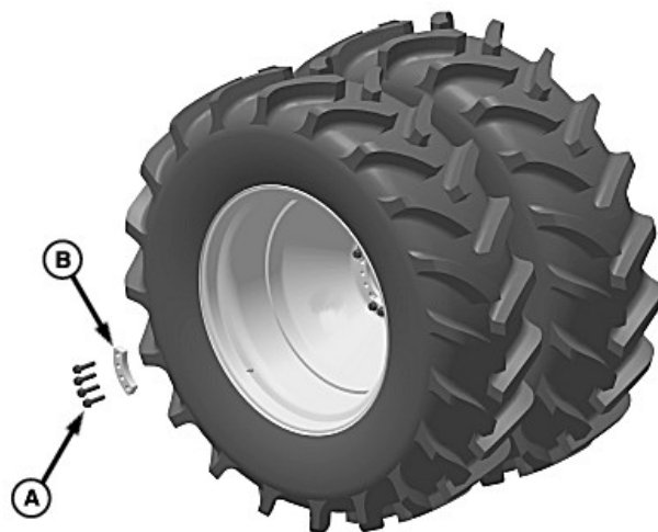
A—Wheel Bolt (20 used) B—Segmented Spacer (5 used)
