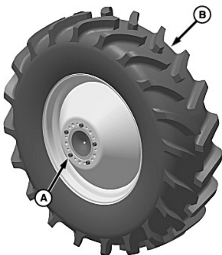
A—Socket Head Cap Screw (5 used) B—Inner Wheel Assembly
